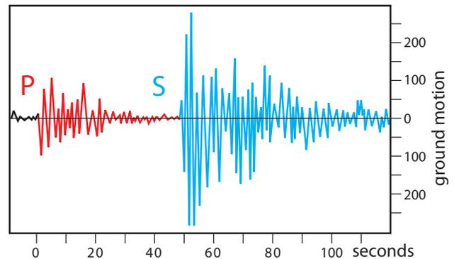
Seismographs create seismograms, which are graphs depicting ground motion. This seismogram is for an earthquake about 350 kilometres away (showing P and S waves).
