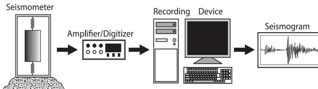
Measuring and converting ground motion into a readable graph (seismogram).
